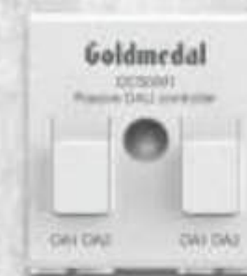
DCS0001 is a BLE-enabled DALI controller. It does not have its own power supply. Instead, it is powered directly from a DALI bus. DCS0001 can be used with a DALI sensor for presence detection or daylight harvesting or it can be used for controlling Human Centric Lighting (HCL).
